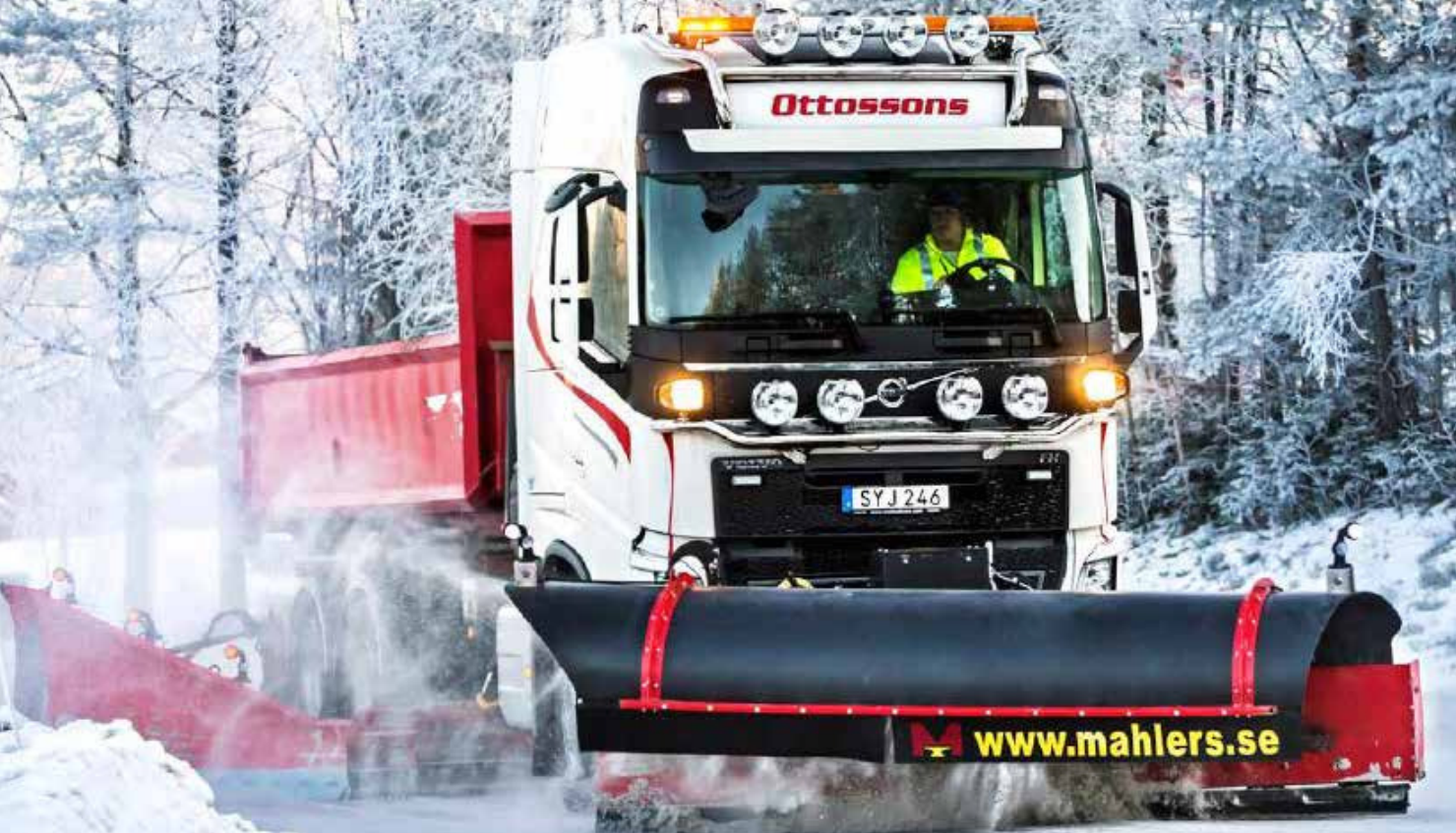
Ottossons newest snow plough, a Volvo FH 6x2, model year 2015, has radar mounted to the front. It looks like a black plastic plate mounted some way down on the grille. On each side of the grille is a new, simpler hitch mounted (see image below). Photo: Michael Engman.
