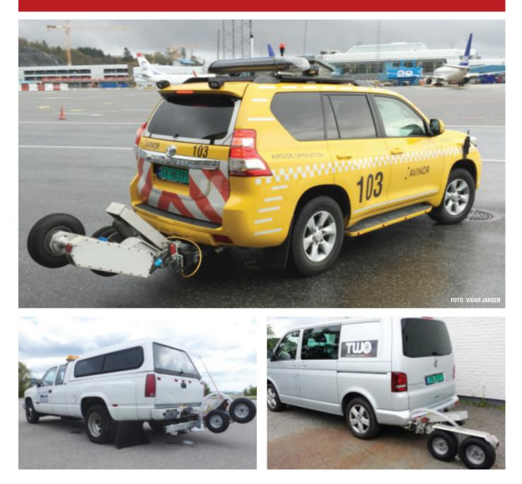
Friction meter using precise weight values for definition of friction. Friction meter with additional equipment that provides exact local knowledge.
